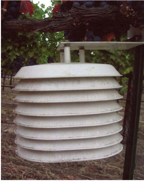
Figure 32 Typical radiation shield for measurement of air temperature. Unlike the state of this shield, it should be kept clean to ensure best alignment with air temperature.
