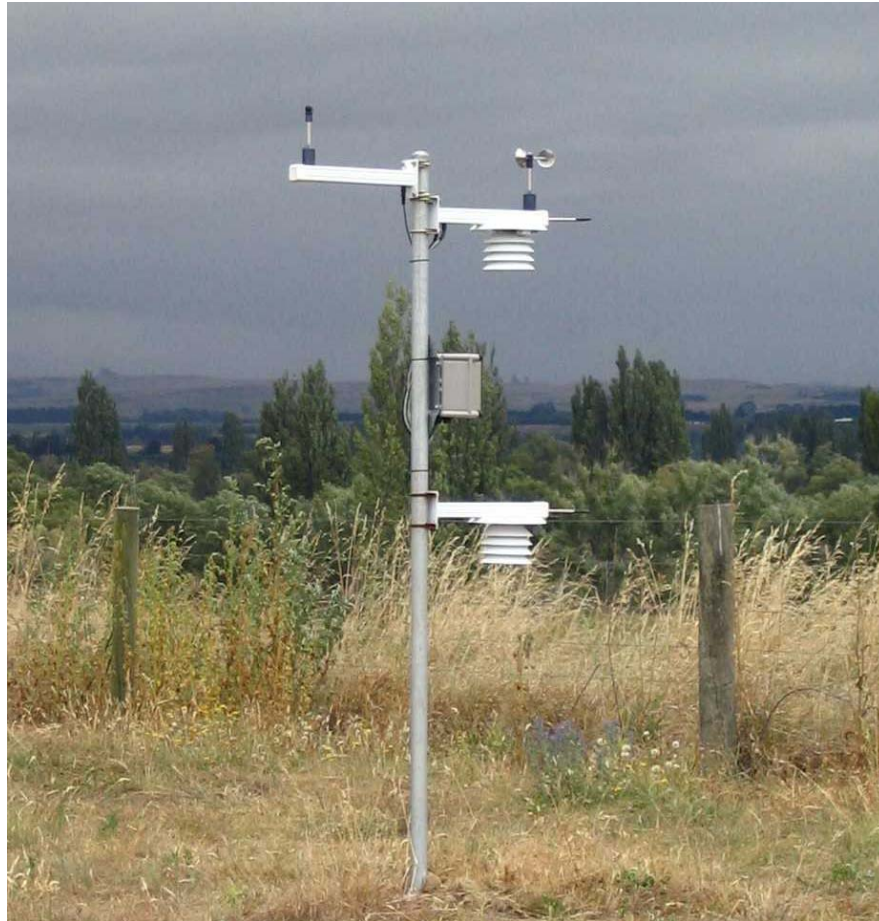
Figure 2 The weather stations comprised a mast for measurements of air temperature, exposed temperature, wind speed and wind direction at two metres, and air temperature, exposed temperature and relative humidity at 1.2 metres (standard meteorological screen height).
